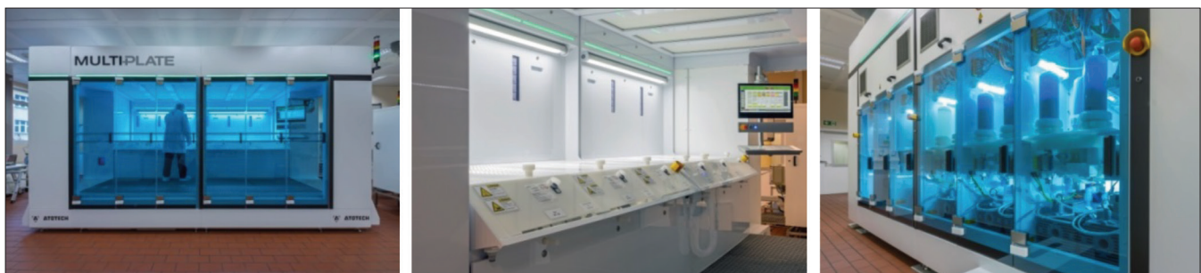
Figure 5: Images of a manual MultiPlate system; (left) front view; (middle) plating baths; (right) chemical distribution units
