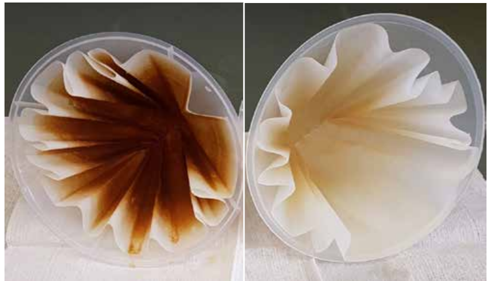
Figure 1: Low Pd precipitation / low sludge formation (11 m 2 /L throughput). Left: Standard activation, right: Neoganth® E Activator System
