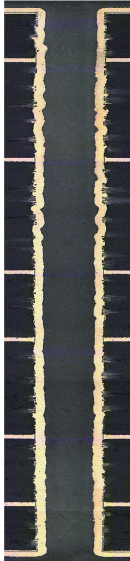
Figure 2: Panel thickness of 4.2 mm, hole diameter 0.3 mm, thro- wing power >90%
