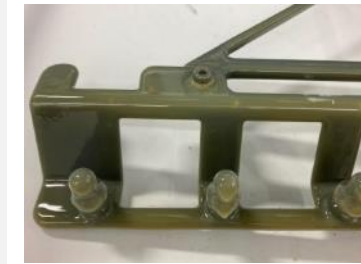
Paint fixture prior to paint removal
