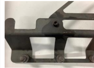
Paint fixture after paint removal
