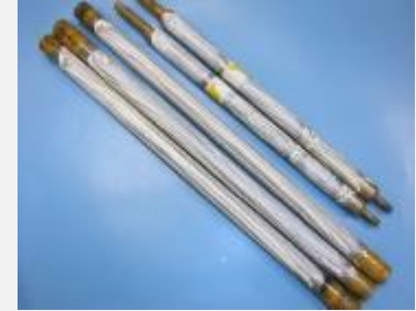
CaCl 2 solution 720 g/l Mix 30g of kolin to CaCl 2 solution Test condition 60 °C, 3 – 8% of humidity, 96 h
