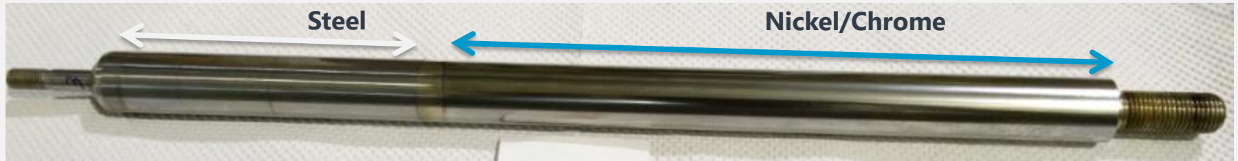
Shock absorber plated with BluCr ® (w/o post-treatment)
