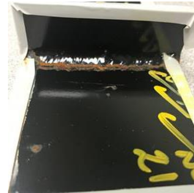
After descaling (840 hours)
