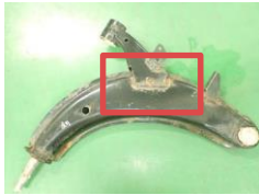
Cyclic corrosion = 50 cycles (1 year)
