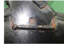
Existing pretreatment + chemical descaling
