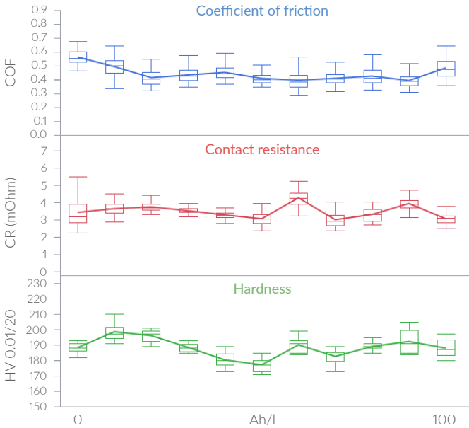
Figure 1: Deposit characteristics of a 35 µm Ag layer for fresh and aged electrolytes
