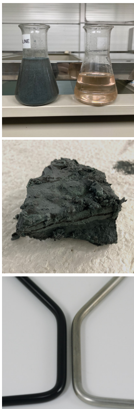
Fig. 1: Master Remover bath Fig. 2: Dry-waste leftover from Master Remover stripping process Fig. 3: Steel fixtures cleaned with Master Remover
