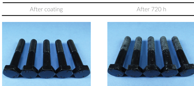
Figure 1 + 2: Surface appearance of Zintek 300 HP + Techseal Glossy Black SL before and after Neutral salt spray test
