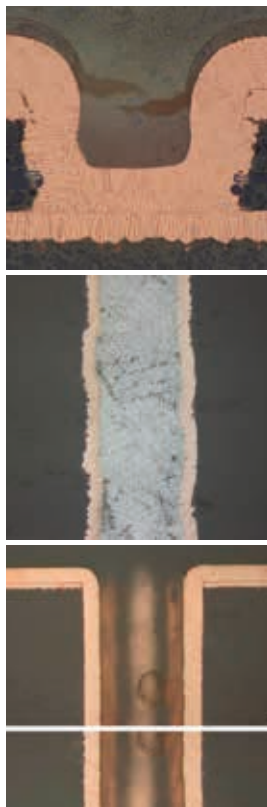
Figure 1: BMV with >80% throwing power at 2.2 A/dm 2
