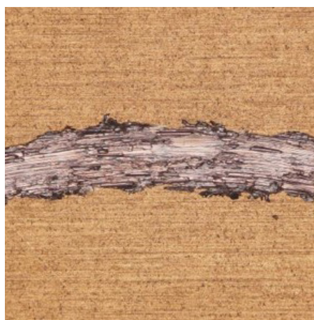
Figure 3: 1.5 \mu\text{m} Ni, 0.3 \mu\text{m} Au plated on Copper base
