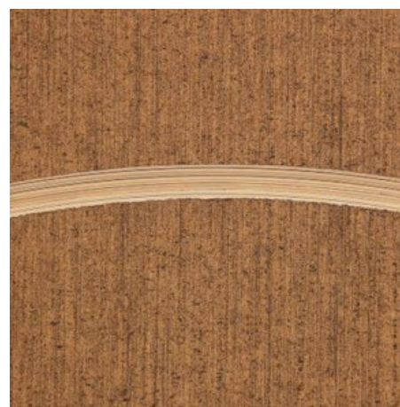
Figure 4: 1.0 \mu\text{m} Ni, 0.6 \mu\text{m} NiW, 0.3 \mu\text{m} Au plated on Copper base
