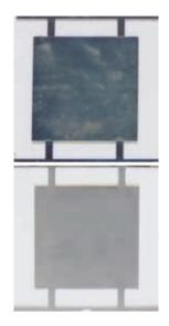
2% K2S immersion test / 5 mins (0.2 μm Ag) with pre-baking @ 200 °C, 1 hour **Figure 1:** Non-treated **Figure 2:** Argalin® XL
